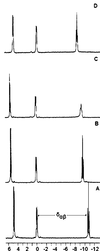
FIGURE 2. 31 P NMR spectra of (A) 5.0 mM Tris-ATP alone, (B) 5.0 mM Tris-ATP with 150 mM LiCl, (C) 5.0 mM Tris-ATP with 0.5 mM MgCl 2 and 150 mM LiCl, and (D) 5.0 mM Tris-ATP with 50 mM MgCl 2 . Trimethyl phosphate was the external reference, and the ionic strength, pH, and temperature were 0.15 M, 7.4, and 37 °C, respectively, in all samples.
